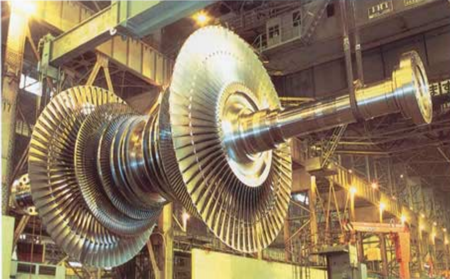
▲ Turbine for power generation
