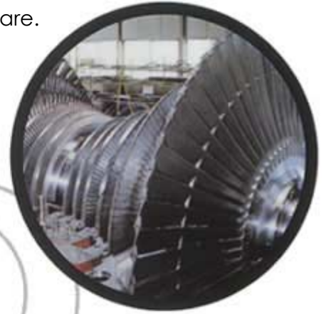
ROTOR FOR STEAM TURBINE
