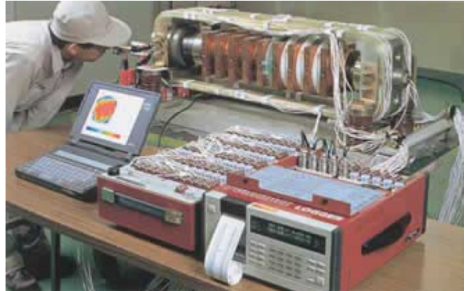
This picture shows the thyristor stack development to study the application technologies of power electronics devices.
