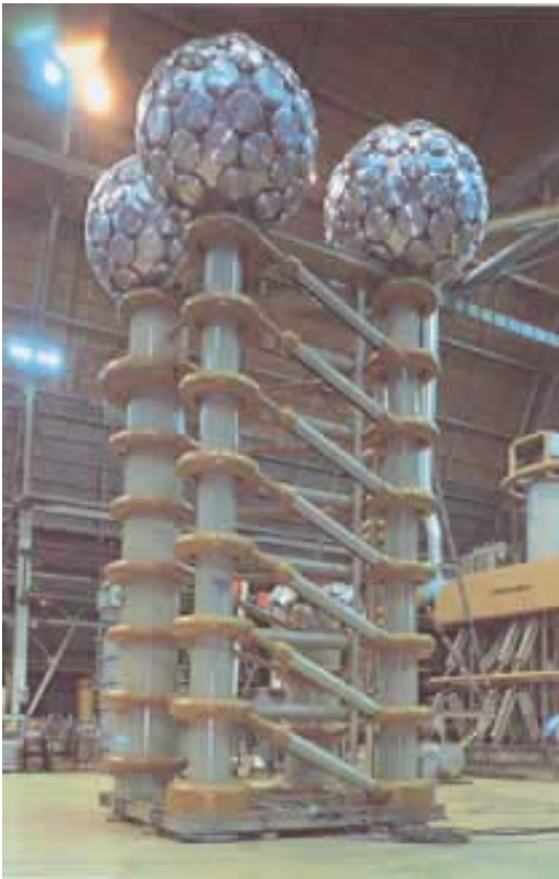
+/- 2000kVDC generation testing facility in the Ultra High Voltage Laboratory is used for the DC high voltage test and the voltage reversal test.
