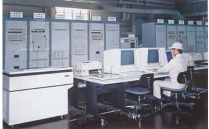
Power system simulator as well as digital analysis using super computers are conducted to evaluate the complex phenomena of the AC and DC systems.
