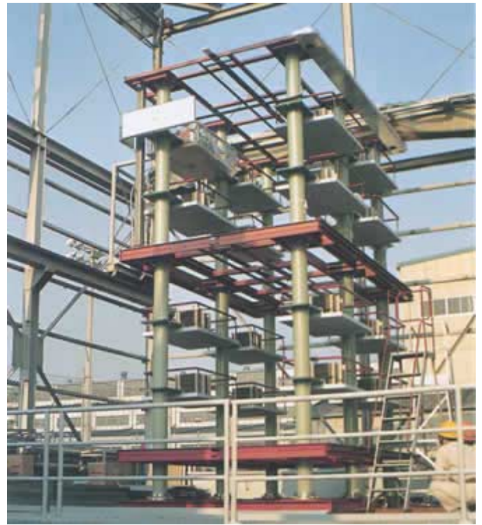
Seismic vibration test of full-scaled quadruple valve
