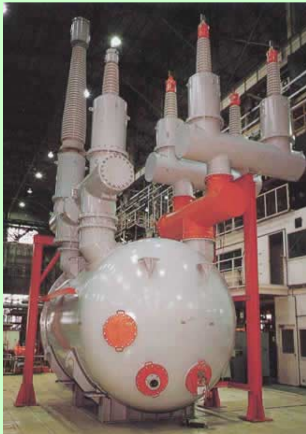
VERIFICATION ON PROTOTYPE TRANSFORMER
