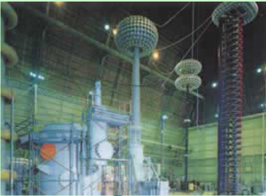
TEST ON FULL SCALE INSULATION MODEL
